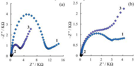
Figure 1. EIS of impregnated graphite electrode (a) and glassy carbon electrode (b); 1 – bare electrode, 2 – gold film surface, 3 – 1-hexanethiol modified gold surface
