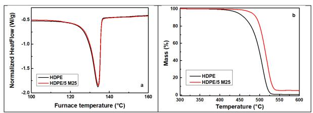
Figure 1. (a) DSC and (b) TGA thermograms for HDPE and its nanocomposite.
