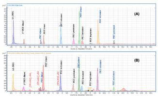
**Figure 1.** UHPLC-QTOF-MS extracted Ion Chromatogram of (A) analytical standards mixture at a level of 0.1 μg kg<sup>-1</sup> 1 for each polyester cyclic oligomer; (B) spiked pasta sample (0.10 μg kg<sup>-1</sup>).
