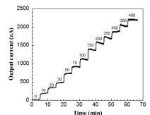
Fig. 1 The response curve of the proposed sensor in glucose solution with different concentrations.
