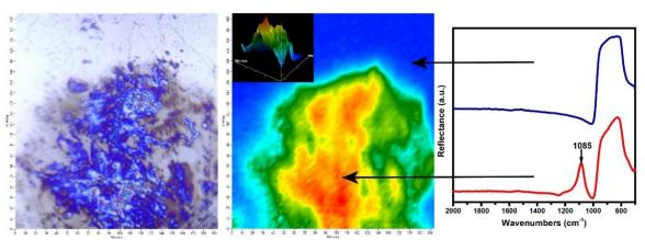
Microscopic image of a SiC surface including unknown superficial spots (left). FPA chemical images using integrated area under Si-O band (centre). Corresponding FTIR spectra of the SiC surface and the  $SiO_2$  spots, the latter as an oxidation product (right).
