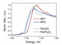
**Fig. 2:** Fe K-edge XANES spectra of potteries and reference compounds
