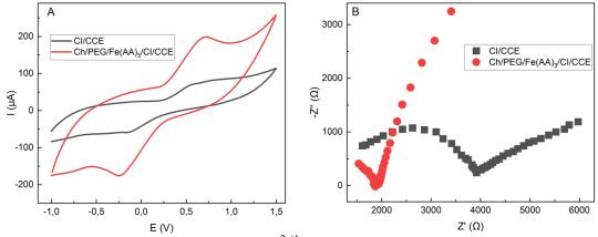
**Figure 1.** A) CVs of 0.1 M  $[Fe(CN)_6]^{3-/4-}$  in 0.1 M KCl at CI/CCE (grey line) and Ch/PEG/Fe(AA)<sub>3</sub>/CI/CCE (red line); B) EIS of 0.1 M  $[Fe(CN)_6]^{3-/4-}$  in 0.1 M KCl at CI/CCE (grey) and Ch/PEG/Fe(AA)<sub>3</sub>/CI/CCE (red).
