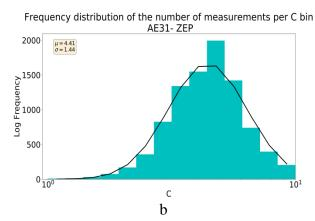
**Figure 1**. a: Zeppelin Station, b: Lognormal frequency distribution of the multiple scattering correction factor for the AE31.
