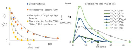
**Figure 1.** Kinetic profiles of (a) diclofenac under different photocatalytic systems, (b) formed TPs under SSL- MOF- $H_2O_2$  system
