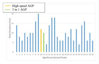
Figure 1. Significant aerosol peaks from AGPs in the first study
