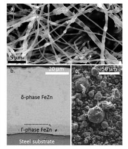
**Figure 2.** SEM images of a. bioactive polymeric-ceramic membranes b. anticorrosion coating (cross-section) and c. thermoelectric MnSi powder obtained using the JEOL JSM-7610F Plus Field-emission SEM recently installed in AMDe Laboratory<sup>1</sup>.
