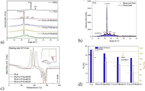
**Figure 3.** X-Ray Diffractograms of PHSu, PLA and their copolymers (a), Fitting profile of PLA (b), DSC heating thermograms of PLA and its copolymers(c), Xc by DSC and XRD against Tcc in the form of columns (d).
