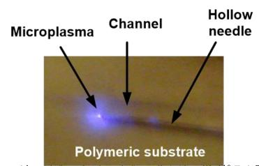
Figure 1. The microplasma (above) is formed at the end of a needle (with an ID=110  $\square$ m). The needle is offset from the microchannel for illustration purposes. The channel is covered using a flexible, polymeric substrate (e.g., 0.3 mm poly carbonate plate).
