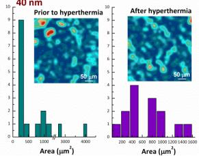
**Figure 1:** Distribution of  $15x15 \mu m^2$  inclusions of MNPs having a mean diameter of 8, 10 and 80 nm, respectively. The  $\mu$ -XRF maps used for the former calculations are shown in the inset (map dimensions are  $450 \times 450 \mu m^2$ , step size is  $15 \mu m$ )
