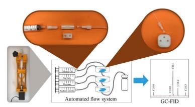
Figure 1. Automated 3D printed flow system for the transesterification of triacylglycerols in edible oils.
