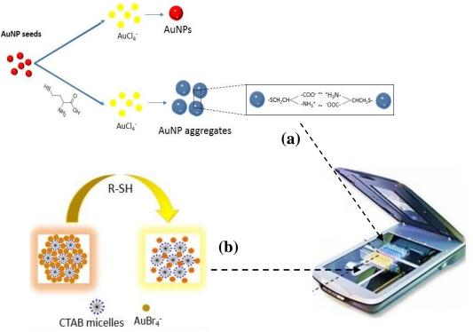
Graphical representation of the potential mechanisms of biothiol sensing based on (a) the effect of biothiols on the growth and aggregation of gold nanoparticles and (b) gold-coated CTAB micellar assemblies.
