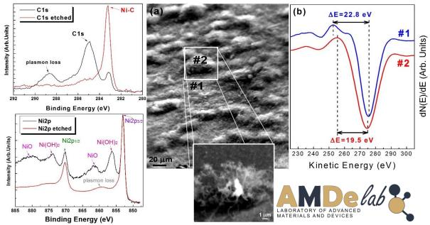
HR XPS measurements of nanocomposite catalysis of DLC: Ni for the growth of CNTs before and after the Ar Ion etching of the surface (at left). (a) FEG AES measurements and quality tests of CNTs on two different spots as shown in the SAM images. Spot #1 indicates an excellent quality of CNTs because of the nano-scale Ni particles as a substrate for the growth of CNTs. Spot #2, on the other hand, shows bad quality CNTs. (b) AES spectra from the two spots.
