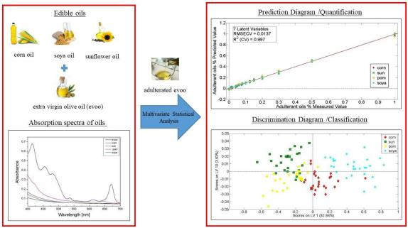
Figure 1. Absorption spectra of different types of oils and the exported multivariate statistical analysis diagrams
