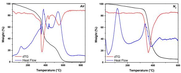
**Figure 1**: Thermogravimetric curves (weight loss, dTG and heat flow) of the epoxy/catalyst mixture, under air (left) and nitrogen (right) atmosphere.
