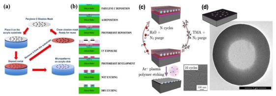
**Figure 1.** (a) Sequence of steps for micropatterning using reusable parylene C shadow masks and (b) sketch of the fabrication steps used to obtain the parylene C stencils. (c) Scheme of the sequential infiltration synthesis of BCPs cylindrical nanotemplates and SEM image of the resulting metallic oxide replica. (d) Microtemplate on silicon used to direct BCPs' self-assembly in the Dekati pattern.
