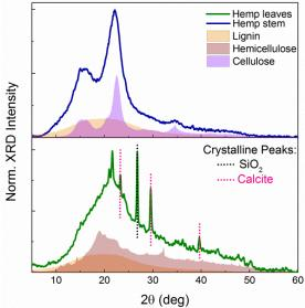
Figure 1. XRD diffraction patterns of feedstock obtained using the Rigaku Ultima Plus X-rays diffractometer placed in the AMDe Laboratory¹ of Physics Department of the Aristotle University of Thessaloniki.
