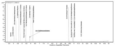
Figure 1. GC-MS chromatogram of spiked food simulant A (10 % v/v) ethanol in water
