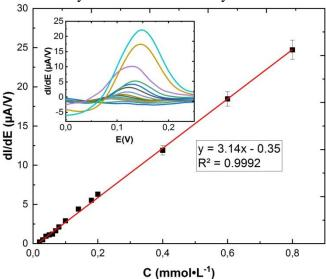
**Figure 1.** Dependence of the cathodic current on IMGE in the first derivative mode of 2,3-dichloro-1,4-naphthoquinone on its concentration in ethanolic solution of 0.1 M NaClO<sub>4</sub> (pH 2.0. potential scan rate 100 mV·s<sup>-1</sup>.
